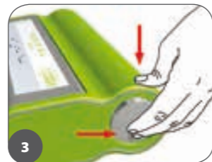
Figure 3: First push with the wrist on the top of the machine (at the same place as when locking), and then press against the inside round plate with the fingers, which is on the side of the machine.
